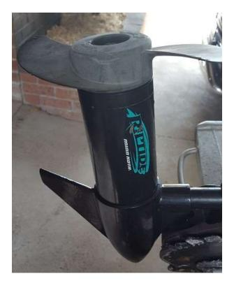
I brought my saltwater electric secondhand about ten years ago, and after each outing I cleaned the motor down to remove all saltwater and gave it a light spray of CRC226 which helps remove any residue.
