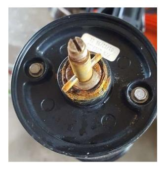
Removing the pin that spins the prop took about half an hour as it was rusted into the shaft, copious amounts of lubricant and a  $1/8^{\text{th}}$  pin punch and finally it came out.
