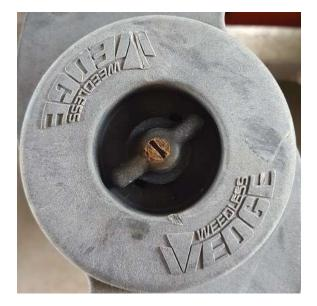
Upon removal there was clear evidence of rust around the shaft so I felt justified that I was on the right track with the overhaul.
