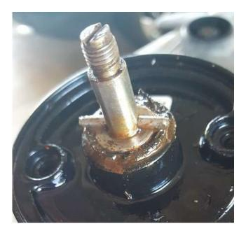
Prior to removing the stator (the big outside round bit) I put a small mark on the body so I could align it on reassembly to the correct position.
