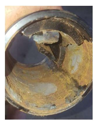
The culprit it would seem is the front seal (adjacent), which was located between the stator and front body, as you can see the bottom of the seal shows evidence of moisture ingress, and that's all it took.
